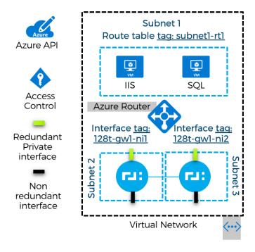
The network interface of the 128T HA router facing the backend applications (e.g. IIS, SQL) is redundant. In the event of a failure of any of the 128T nodes/instances or in the event of a redundant private interface changing its operational state to down, the 128T cloud HA solution will update the Azure router to the healthy node and healthy redundant private interface available, allowing the backend applications to continue to operate normally.
