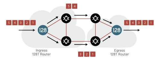
When traffic volume exceeds the bandwidth of the primary connection, the excess is offloaded to the next alternate path. The ingress router is configured by the administrator to use the primary path. When traffic exceeds the bandwidth of the primary connection, the excess traffic is offloaded to the next alternate connection. The administrator can define the interfaces that are being combined for the purpose of session maximization.
