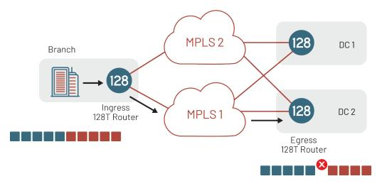
One method for flow performance monitoring is marking of packets in a specific session to different colors, thereby dividing the flow into different consecutive blocks. Packets in a block have same marking and consecutive blocks will have different markings. This enables the measuring node to count and calculate packet loss and/or delay based on each block of markers without any additional OAM packets.
