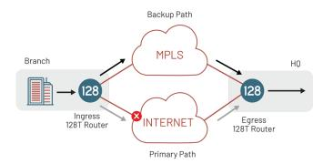
The traffic always flows over the Internet connection. In case of performance degradation, the sessions are moved to the MPLS connection. When the Internet connection is restored to acceptable performance, the sessions are moved back to the Internet connection.
