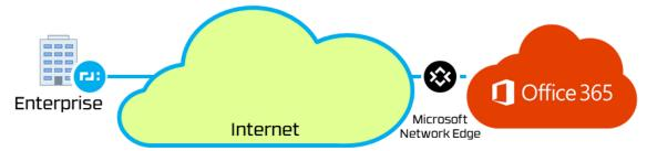
Distributed Internet access is the most popular method for enterprises to connect to Office 365 whose sites are geographically close to a Microsoft Network Edge location. 128T routers deployed in branch locations will enable improved performance and eliminate "tromboning" from any location.
